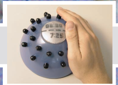
In this alarm clock design, one button stands for a certain amount of sleep. From the way in which the buttons are pushed, the alarm clock can infer the importance of waking up and vary its sound accordingly (design: H. Hellman and L. Ypma).
