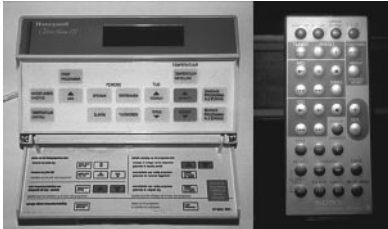
Digital products are generally controlled by buttons and icons, an approach which emphasises the user's cognitive skills. Examples of such interfaces are a Honeywell thermostat (left), a remote control for SONY hi-fi equipment (right)
