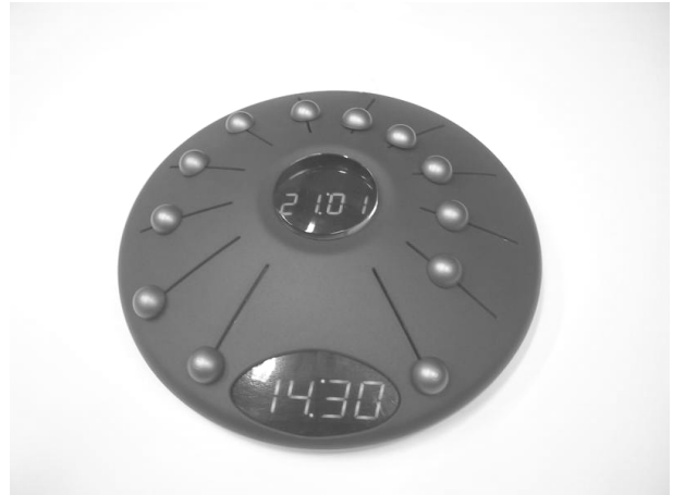
Fig. 5 The working prototype. The user can set the time by sliding the knobs. And he can do this in many different ways, thus expressing his emotion
