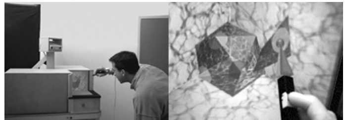
Fig. 1 The head movements of the person are recorded. A computer generates 3 images, corresponding with the person's viewpoint, and projects them on 3 orthogonal screens (left). The person sees a 3D object and has a hybrid instrument with which he can interact with this object (right).
