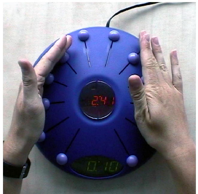
Figure 1: The prototype of the alarm clock
