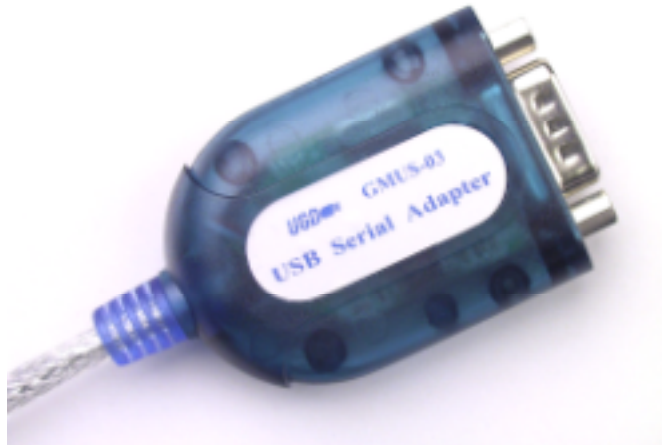
Figure 2: GMUS-03 USB-serial adapter
