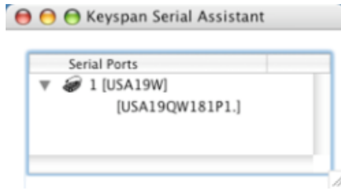
Figure 5: The Keyspan Serial Assistant acknowledges the adapter
