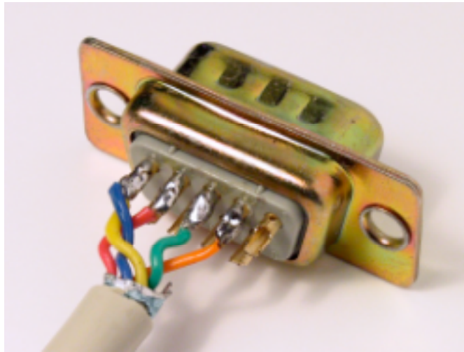
Figure 10: The finished soldering job on the DB9 plug
